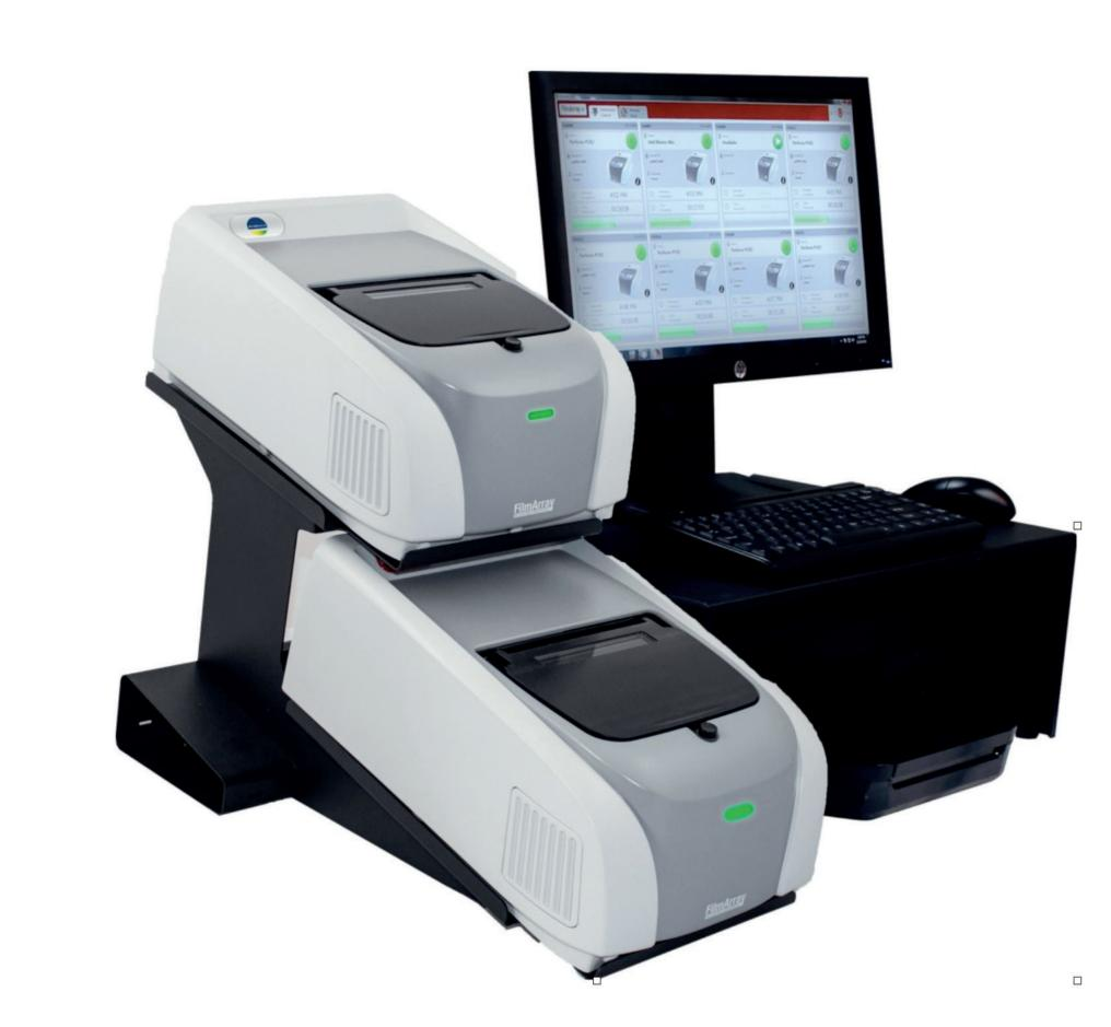
**Figure 1:** FILMARRAY 2.0 Industry instrument performs the extraction, amplification and detection (25.4 x 39.3 x 16.5 cm/10 x 15.5 x 6.5 in WxDxH). The system comes standard with 2 instruments; up to 8 instruments can be connected to a single PC.
