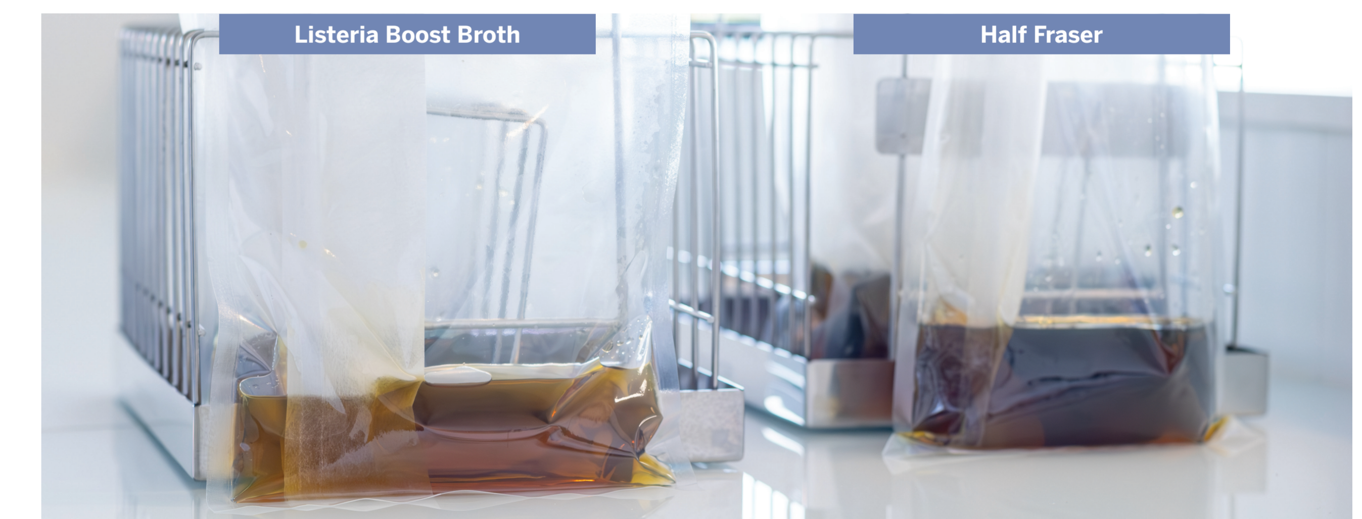
Figure 3: Illustration of the 40% volume saving with new ALOA® ONE DAY short protocol (on the left).
