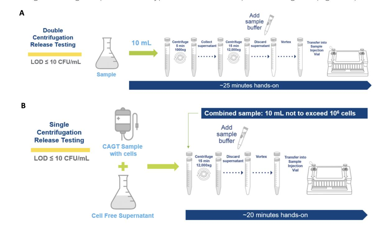
Figure 3: BIOFIRE FILMARRAY 2.0 Industry system release protocols for Mycoplasma testing. A. Double centrifugation and B. Single centrifugation.
