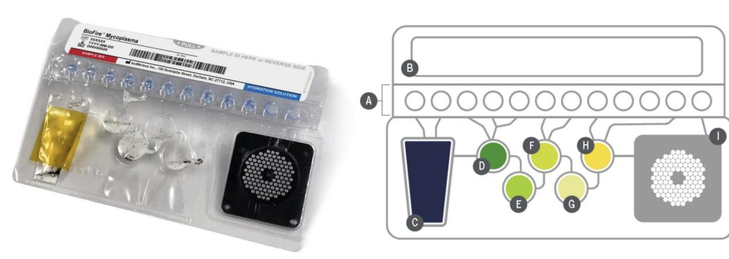
Figure 2. A. BIOFIRE Mycoplasma pouch. B. Pouch diagram A. Fitment with freeze-dried reagents B. Plungers-deliver reagents to blisters C. Sample lysis and bead collection D. Wash E. Magnetic bead collection blister F. Elution G. Multiplex Outer PCR blister H. Dilution blister I. Inner Nested PCR array.
