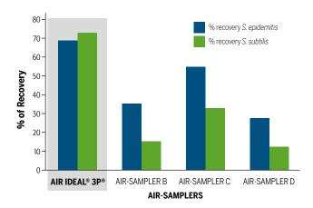
The air IDEAL® 3P® was shown to be able to collect aerosols of Staphylococcus epidermidis with a high efficiency of 92.1%.
