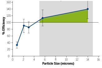
The result of physical evaluation of AIR IDEAL® 3P® following the ISO 14698-1 standard, demonstrated that the bioMérieux air sampler is highly efficient for collecting particles containing bacterial cells in the range 2.1-14 microns.
